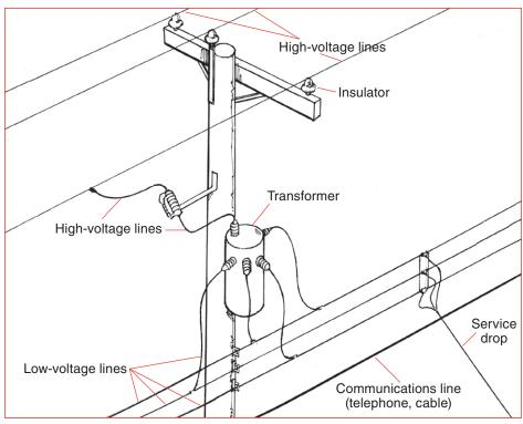
Overhead electrical conductors can often be identified by their placement on the pole.
