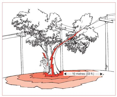
If anything touches a high-voltage power line or if a power line falls to the ground, electricity will flow to the ground, energizing the tree or equipment and anything in contact with it. The surrounding ground may be extremely hazardous. The voltage gradually decreases from the point of contact until it reaches zero. The safe distance shown here—10 metres (33 ft.)— is for line voltages up to and including 60 kV (60,000 V).
