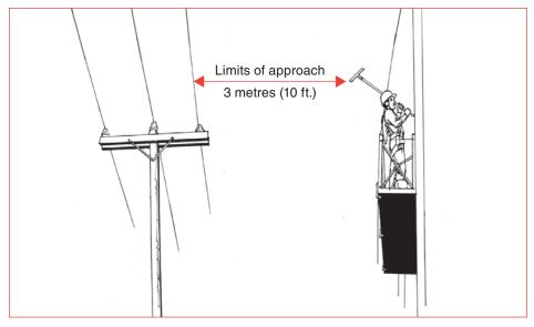
The tool is an extension of the worker's reach and must not come within the limits of approach.
