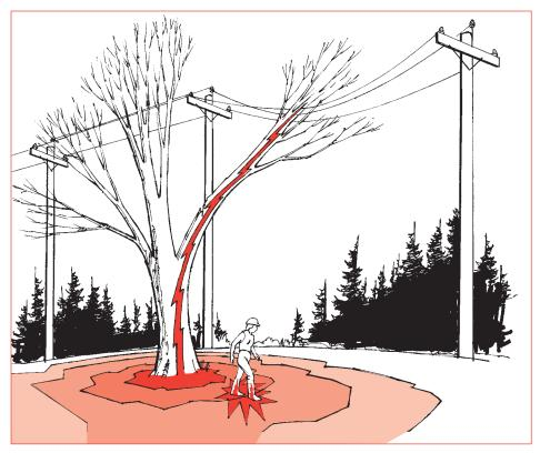
Step potential: If your feet are spread apart on energized ground, electricity can flow through your body from the area of higher voltage to the area of lower voltage.
