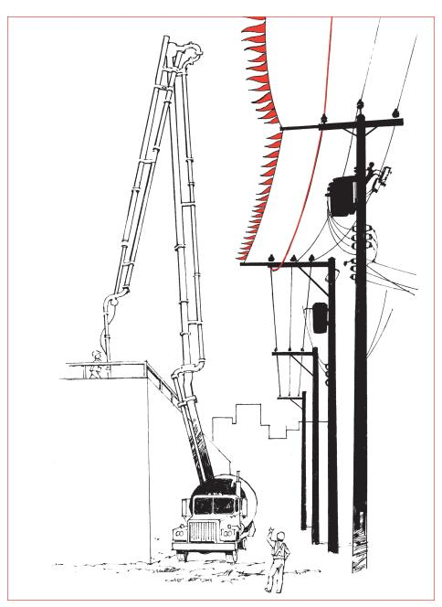
Guarding is a visual warning only. The grounded guard wire (with flags) gives warning of approach. The overhead line cover-up, installed by the owner of the power system, has no insulated rating for the purposes of Form 30M33. Workers and equipment must not contact the guard wire or overhead line under any circumstances.
