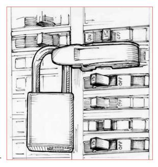
Lockout is required at the electrical panel before replacing any part associated with the lighting circuit. For testing of lighting circuits prior written permission is not required from WorkSafeBC as long as the testing is done using established safe work procedures and using test equipment and tools that are CSA approved.
