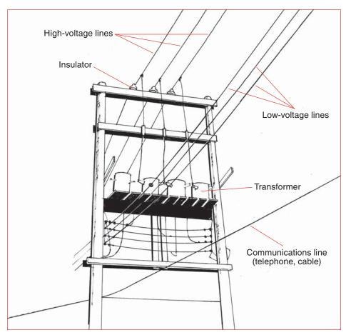
An H-frame configuration may be used to facilitate the installation of transformer bank platforms on older systems. They are most often seen in alleys. The illustration on page 4 shows a common single-pole configuration.
