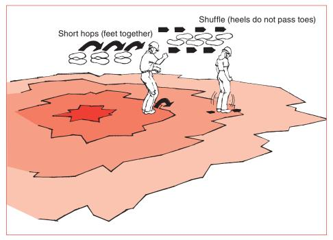
If you must move on energized ground, shuffle or hop while keeping your feet together and touching each other. Do not take steps.
