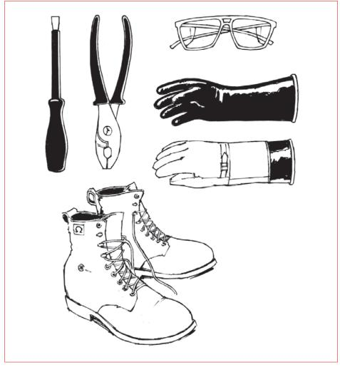
When working on energized low-voltage equipment, workers need protective equipment, including insulated tools, safety eyewear, rubber gloves, and shock-resistant footwear.
