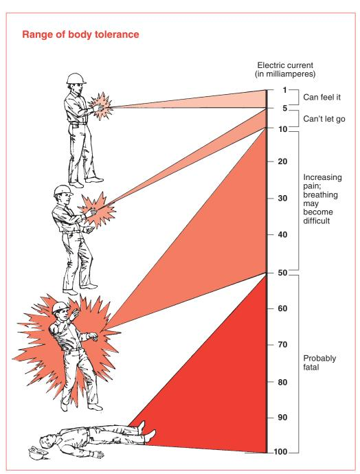
A 100-watt light bulb uses 1000 mA (milliamperes) of current. It takes only 5 mA to trip a ground fault circuit interrupter (GFCI). A small amount of current running through the body for a few seconds can give the effects shown in the table.
