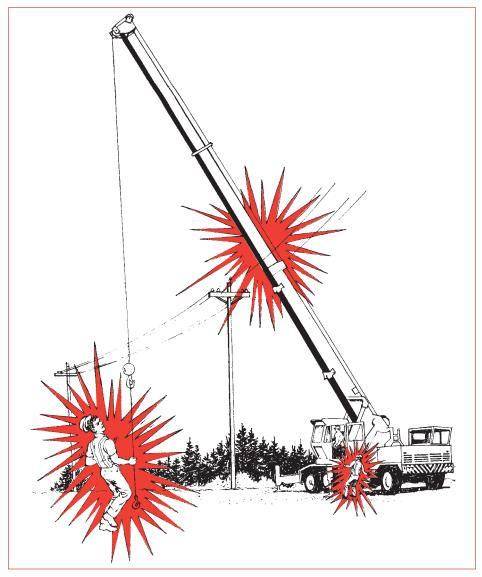
If mobile equipment touches a power line, electricity can travel from the power line to a worker touching any part of the equipment, including a pendant control.
